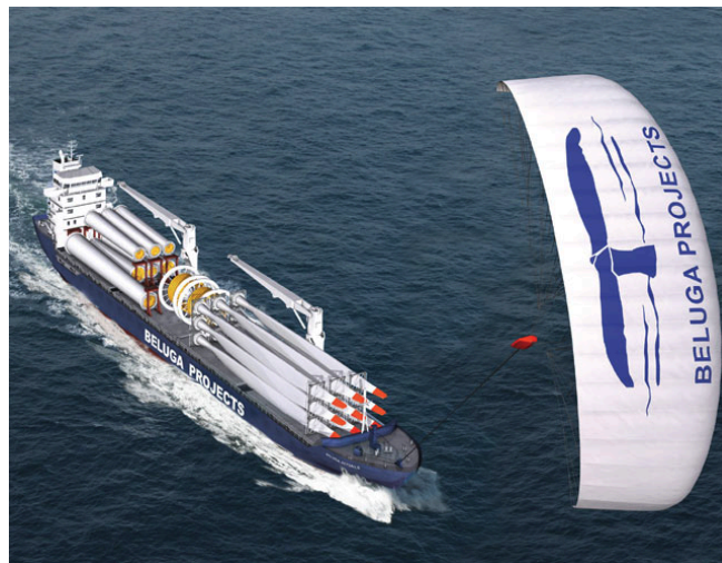
Kite sail providing supplemental power to the MV Beluga Skysails
