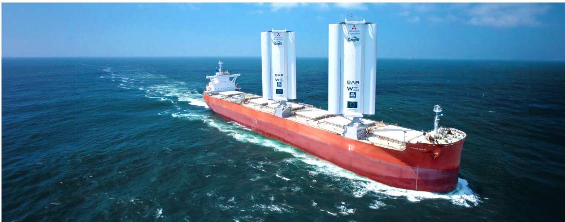
WindWings—wind powered cargo ships—were designed within a partnership between Cargill, BAR Technologies and MC Shipping. Photo Courtesy of Cargill
